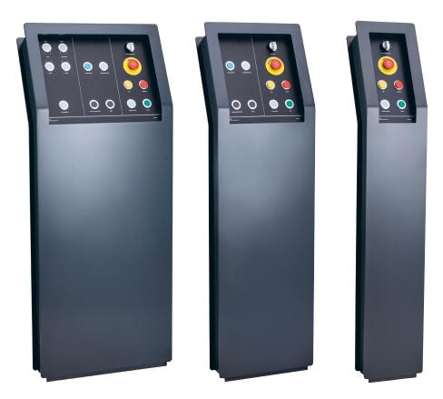
The newly developed control system places the emphasis on the needs and tasks of the user. From the central control desk, you have a full overview of the ropeway installation and can simultaneously keep an eye on your passengers. The premium touchscreen is ergonomically angled and made of top-grade materials.
